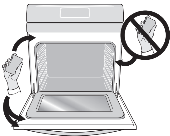
Figure 21: Clean around the oven door gasket
